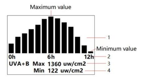
At the bottom of the chart, there are two numerical indicators: Max and Min. The Max and Min values will reflect the maximum and minimum values on the chart of UVA+UVB intensity.
