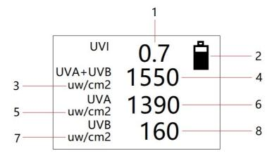
**Note:** If the UVs radiation intensity exceeds 9,999uw/cm2, the units will switch to mw/cm2. 1mw/cm2=1000uw/cm.
